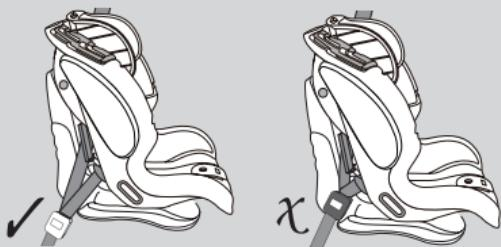
With your child car seat now buckled in, check it is secure by pulling forward from both harness straps, there should be little or no movement. Next check that the vehicle's seatbelt buckle is NOT resting against the child car seat shell. This is called 'buckle crunch' and could cause the child car seat to work loose or the seatbelt to come undone in an accident. If you find you are experiencing 'buckle crunch' then this child car seat is not suitable for your vehicle.
