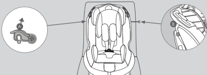
Release catch (A) on the top left hand side of the shell and remove the installation bar (B).
