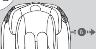
Release catch (A) on the top left hand side of the shell and remove the installation bar (B).
