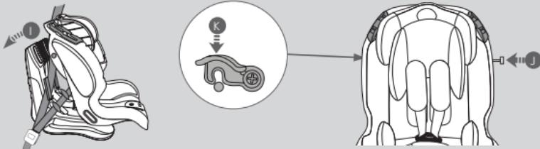
Return the shell to its original position (I) (taking care not to trap the diagonal shoulder belt) and thread the installation bar back through the seat (J). Secure the catch on the top right hand side of the child car seat (K). Pull the installation bar to ensure it is securely locked in place.
