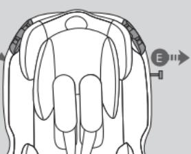
Release catch (D) on the top left hand side of the shell and remove the installation bar (E).
