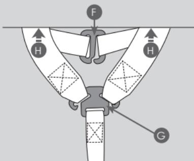
Unhook the shoulder pad straps from shoulder pad connector (F). Unhook the shoulder harness straps from yoke (G). Pass the shoulder straps through the slots in the back of the shell (H).
