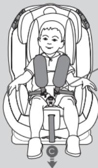
After placing your child in the child car seat, match the two halves of the harness buckles together and insert them into the crotch buckle. Make sure the shoulder straps fit your child snugly by pulling the adjuster belt (C).
