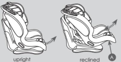
The child car seat can be used in four different seat positions, from seated to a reclined sleeping position. Pull the recline adjuster handle (A) under the front of the shell and pull the shell forwards or backwards, release the handle on your required position when hearing a distinct click.
