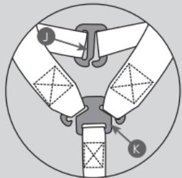
Connect the narrow shoulder pad straps to the shoulder pad connector (J). Connect the wider shoulder harness straps to the yoke (K).
