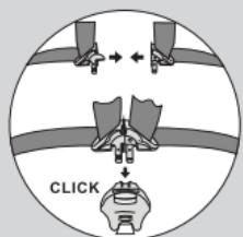
Take the two harness shoulder straps with the buckle clips and crotch strap and match the buckle tongue sections together and insert into the buckle.
