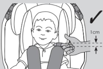
The harness should allow 1 finger-width (1cm) of space at the top of the shoulders. This is the ideal tightness.
