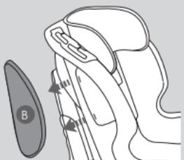
Pull the two (SAP) Side Armour Protection systems (B) in the direction of the arrows to unclip them from the shell and remove their covers.
