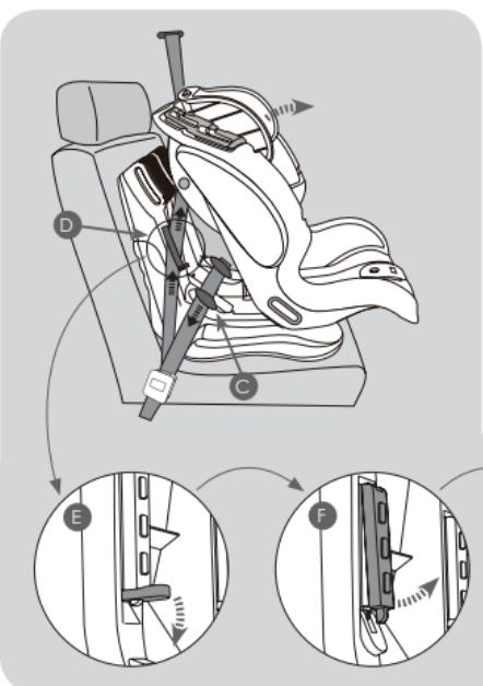
Push the child car seat back into the passenger seat ensuring a good fit. Thread the horizontal lap belt section under both hooks (C) and remove all the slack by pulling up on the diagonal section of seatbelt. Thread the diagonal section through the lock off device (D) that is nearest to the seatbelt.
