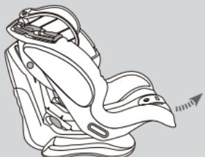
Pull the recline adjuster handle under the front of the shell and whilst holding it, pull the shell forwards to its most reclined position.
