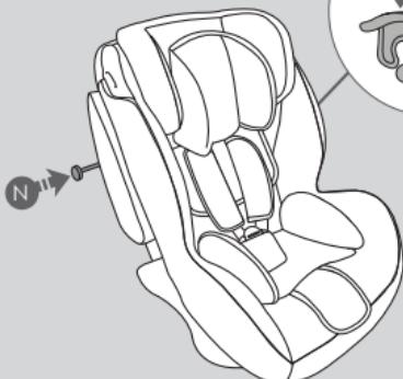
Return the shell to its original position and re-insert the installation bar (N) and secure the catch (O).
