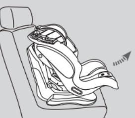
Place the child car seat on a suitable passenger seat. Pull the recline adjuster handle under the front of the shell and adjust the shell to its fully reclined position.
