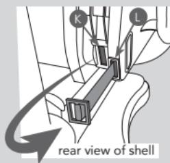
Locate the two metal retainer buckles (J) under the seat cover at points (1) and (2). Pass the metal buckles on the waist harness from the front of the shell, through the inner slots (K) on the back of the shell and back out the outer slots (L), to the front to remove the harness.
