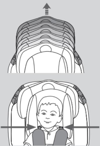
Adjust the headrest by pulling the adjuster handle on the back of the headrest and raising or lowering according to your child's height.
